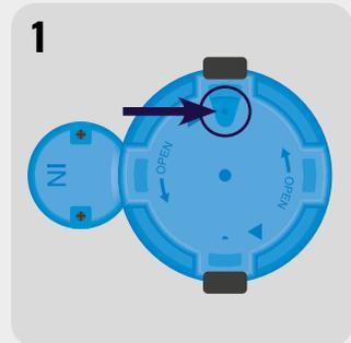
If there was no air trapped, it could be that one of the two internal filters is blocked. First, remove the Activated Carbon Disc (see page 9) and then use your Wayfarer™ again. If it works normally now, you can either fit a new Activated Carbon Disc or continue using your Wayfarer™ without one. If removing the Activated Carbon Disc made no difference, it could be the UF Cartridge has blocked and it may need cleaning or replacing (see page 8).
