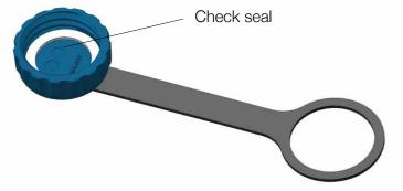
4. Remove vent cap and make a visual check of the flat seal. Check for any splits/cracks etc. Replace as necessary.
