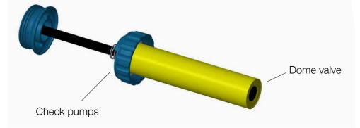
5. Check operation of hand pumps are smooth and fully functional. Remove the pumps and visually check and externally clean the pumps. Replace the dome valve with parts from the spares kit as a matter of course. If there are any defects with the pumping mechanism replace the complete pump assembly.
