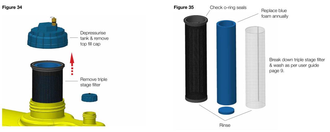
3. Release all pressure. Remove the top fill cap and extract the triple pre-stage filter. Back wash the debris basket and mesh liners with clean water to remove any algae and mildew. Replace with new blue foam pieces. Check both o-ring seals on the debris basket for any splits/cracks etc. Replace as necessary.
