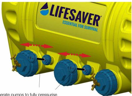
Operate pumps to fully pressurise tank & witness PRV releasing.
